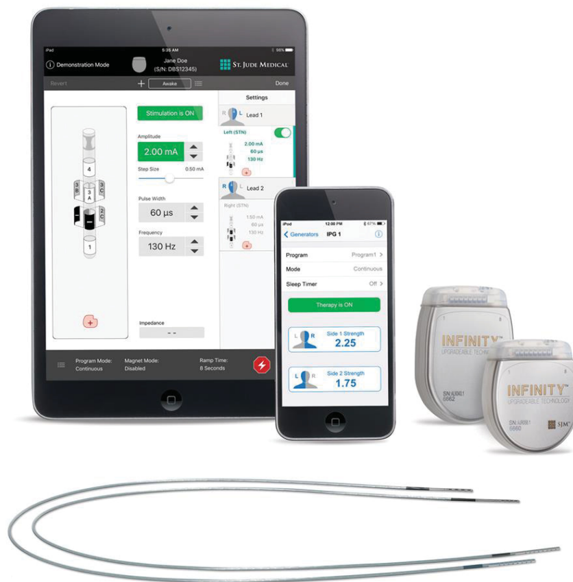
Figure 4: Remote programming device, subcutaneously implantable pulse generator, and electrode wires. The figure was created by Abbott Medical™ and is presented here after an explicit permission.
